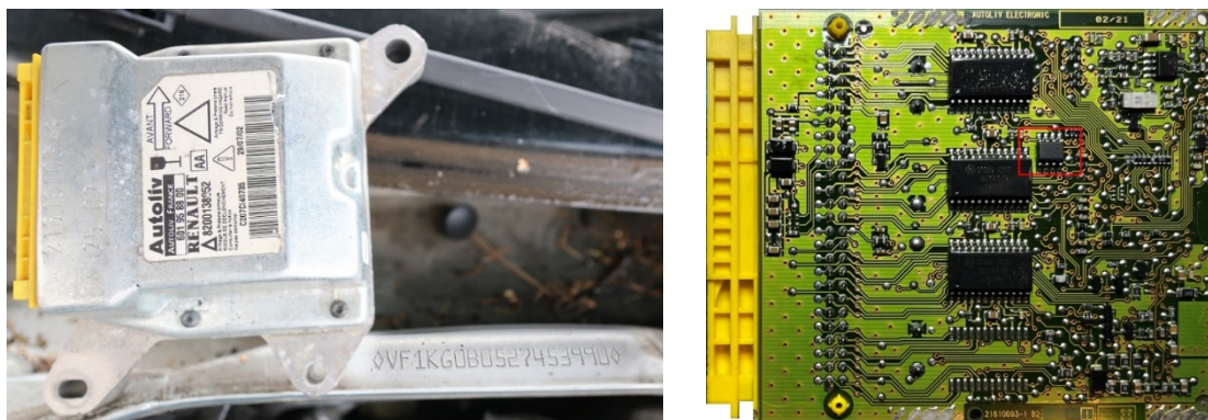
Obr. 18 – Sterownik SRS samochodu Renault i wydobyta z niego płyta. Fig. 18 – The SRS controller of the Renault car and the board extracted from it.
